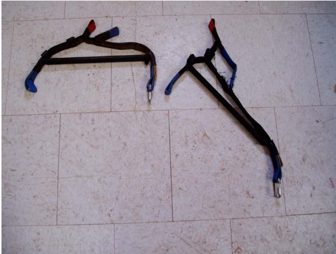
Figure 1 – Normal spreader bar on left, and failed spreader bar on right showing resulting hang position of passenger after failure.
